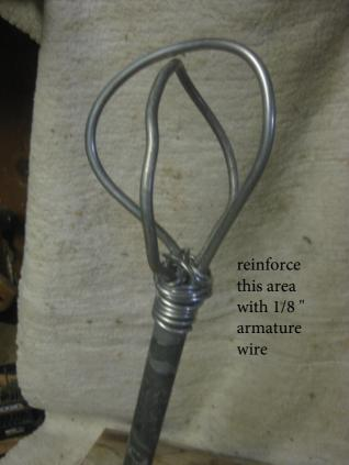
also tie the 2 loops together at the top with 1/4 inch wire add 1/8 inch wire to the loops
